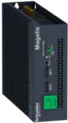
HMIBMO Optimized Box PC, expandable version
