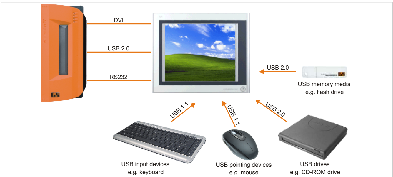
Figure 98: Remote connection of USB peripheral devices on the APC900 via DVI
